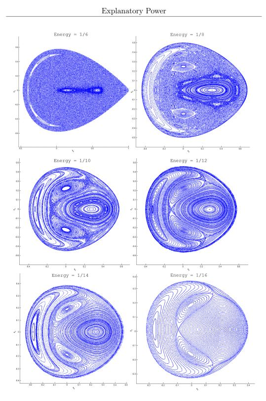
Figure 7: For high energy (E = 1/6), nearly all of the dynamic states are chaotic. As the energy decreases  $(E = 1/8 \rightarrow E = 1/14)$  the regions of chaotic dynamic states shrink, until nearly all dynamic states are regular and predictable (E = 1/16).
