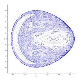
Figure 5: Poincare Map of the Hénon-Heiles system on the  $(q_x = 0)$  plane when E = 1/8
